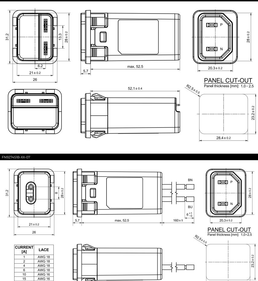
For dimensions [mm] without tolerances: ISO 2768-m / EN22768-m applies
