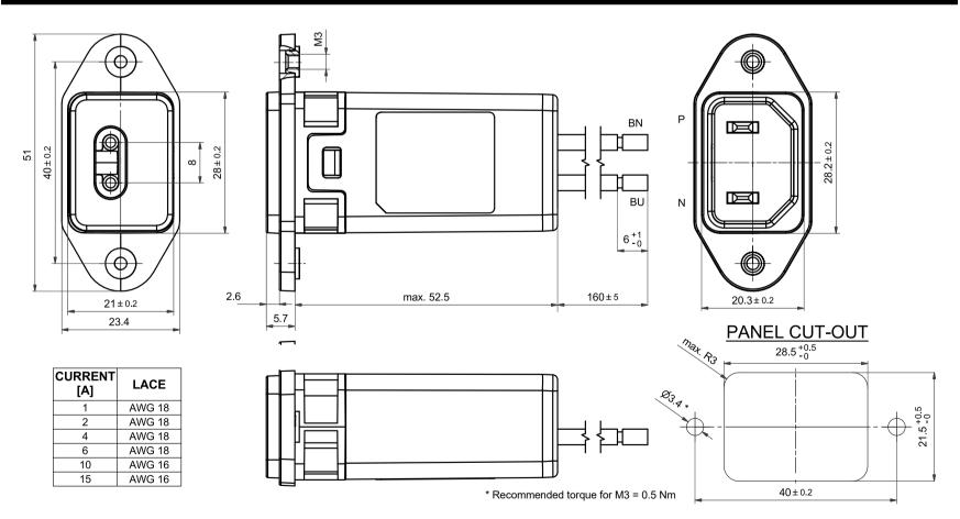
For dimensions [mm] without tolerances: ISO 2768-m / EN22768-m applies
