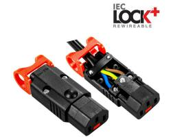
The locking system has a tensile force of typical 300N. It is recommended to use it with flange mount filters. For details refer to our Application Note "Using IEC Lock Power Cords with IEC Inlets
