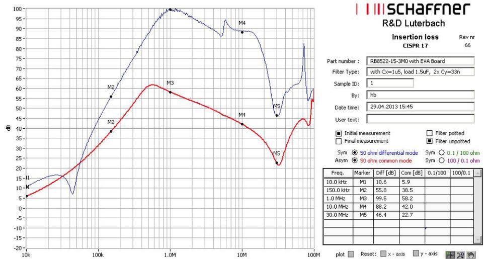
Fig.19: Insertion loss test with RB6522-16-1M0,  $C_x = 1.5\mu F$ , additional  $C_x = 1.5\mu F$  on line side,  $C_y = 33\text{ nF}$
