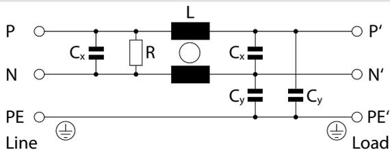
Fig 1: Schematic of a typical single-phase EMC/EMI filter
