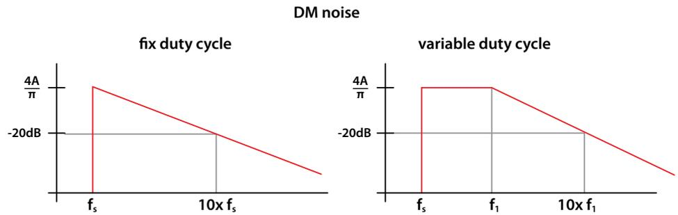
Fig. 9: Simplified envelope curves of DM noise
