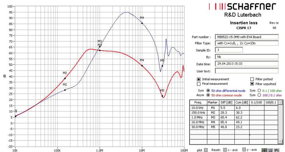
Fig.18: Insertion loss test with RB8522-16-3M0,  $C_x = 1.5 \mu\text{F}$ ,  $C_y = 33 \text{ nF}$
