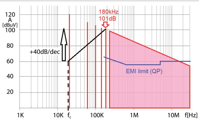
Fig. 12: Principle of EMC/EMI filter design determination
