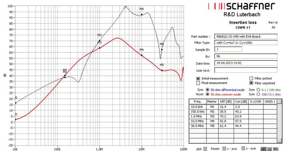
Fig.16: Insertion loss test with RB6522-16-1M0,  $C_x = 4.7 \mu F$ ,  $C_y = 100 nF$
