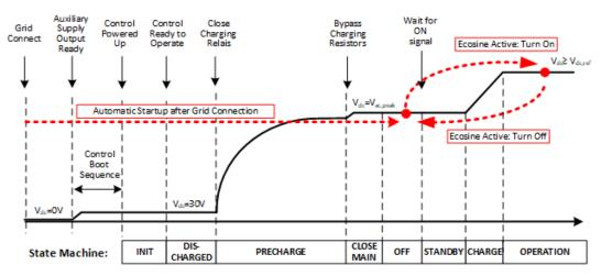
Figure 9-27 Ecosine Active Sync status and DC-link voltage level during startup and normal operation
