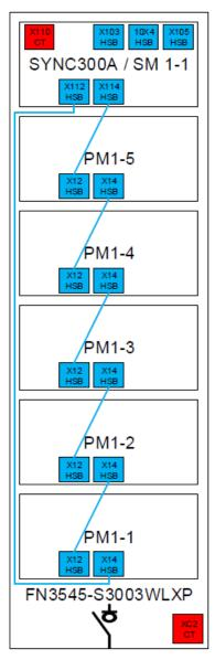
Figure 8-4 HSB connection between sync module and power modules
