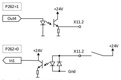
Figure 8-2: Functional connection of digital input/output
