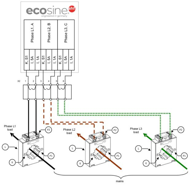
Figure 8-14 CT (1A) wiring for DPP, CTs connected to one module only
