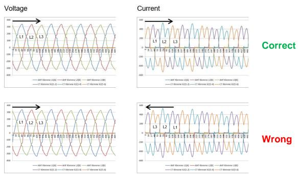
Figure 8-25 Checking rotating field of current and voltage
