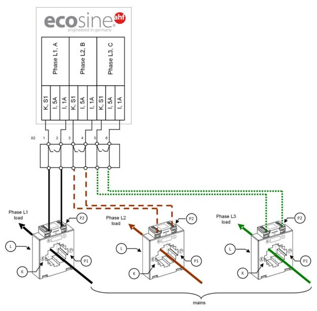
Figure 8-10 CT (1A) wiring for single power module
