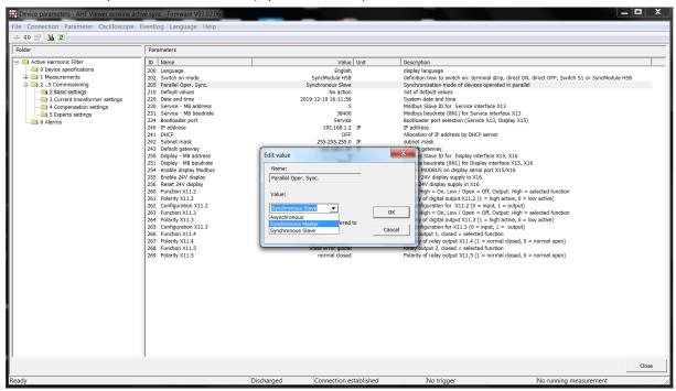
Figure 8-33 Ecosine Active Sync DPP operation Master/Slave configuration.
