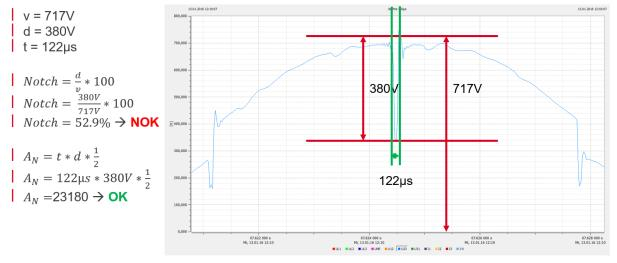
Figure 19-7: Example of notch calculation where notch depth is NOK, while commutation area is OK. These notches are not acceptable.
