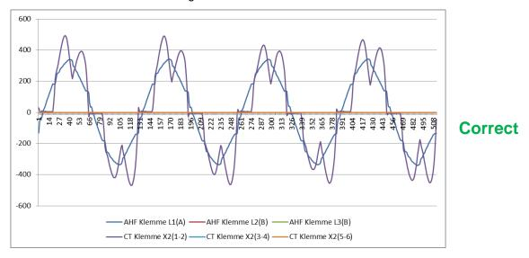
Figure 8-26 Phase of current and voltage is correct
