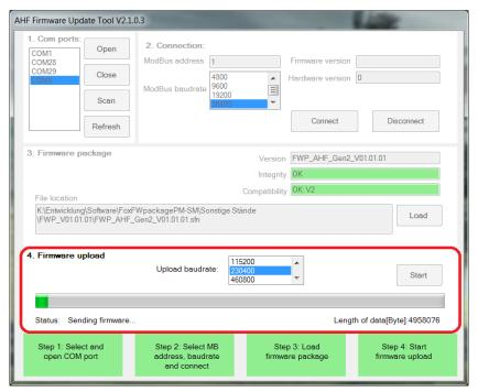
Figure 12-8 Upload of firmware
