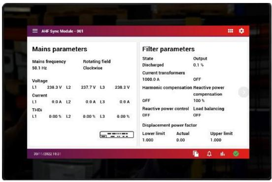
Figure 9-1 HMI 7" touch screen
