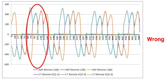
Figure 8-28 Current transformer 1 phase-is shifted through 180°.
