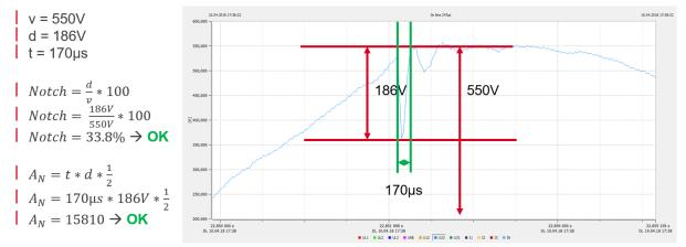
Figure 19-9: Example of notch calculation where both notch depth and commutation area are OK. These notches are acceptable.
