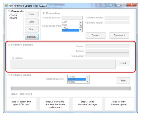
Figure 12-6 Loading the \*.sfn file
