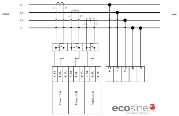
Figure 8-7 Connection of 3-phase 4-wire devices CT secondary output 5A
