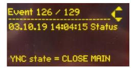
Figure 9-25 Display module screen, events examples
