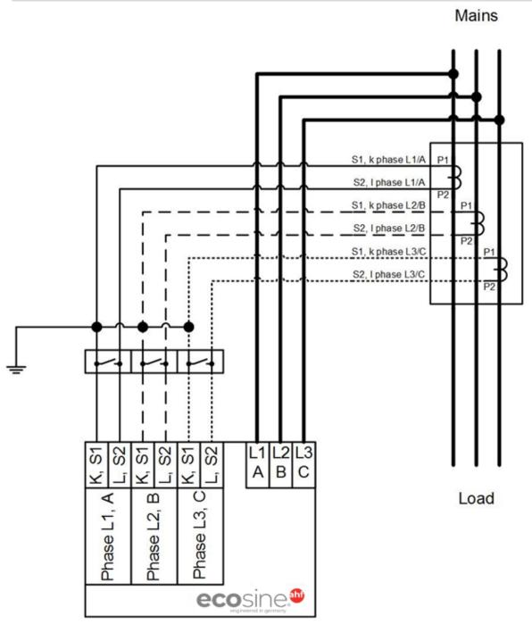
Figure 8-24 Grounding of the current transformers (optional)
