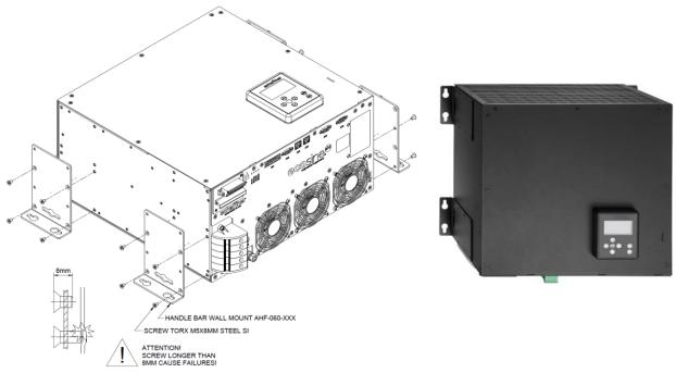
Figure 7-4 Instruction of power module flat mounting
