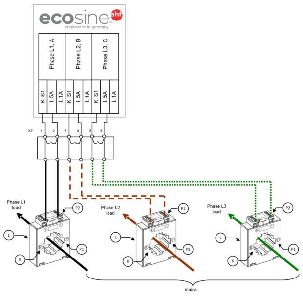
Figure 8-9 CT (5A) wiring for single power module
