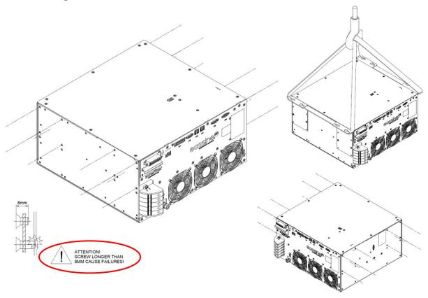
Figure 7-1 Instruction for lifting power module
