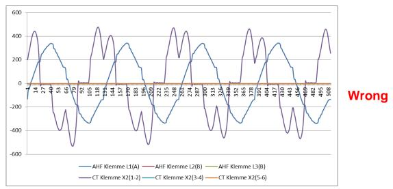
Figure 8-29 Current transformers of phases 1 and 3 are interchanged
