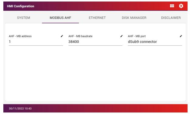
Figure 9-20 Settings menu MODBUS AHF tab
