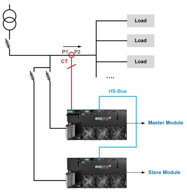
Figure 8-15 CT installation on load side for operation of DPP
