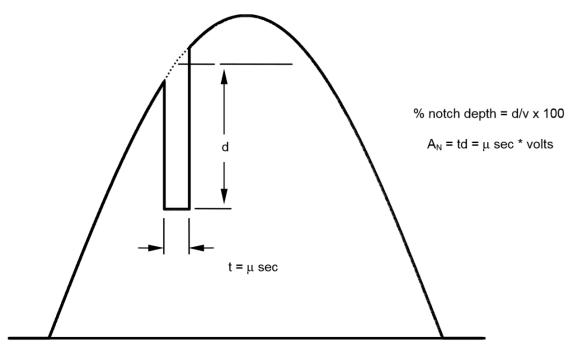
Figure 19-1 calculation of commutation notch area
