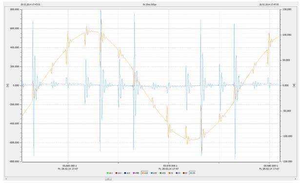
Figure 19-2: Filter current (blue) caused by commutation notches
