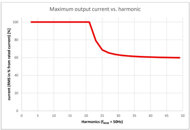
Figure 6-3 Curve of maximum output current vs. harmonics
