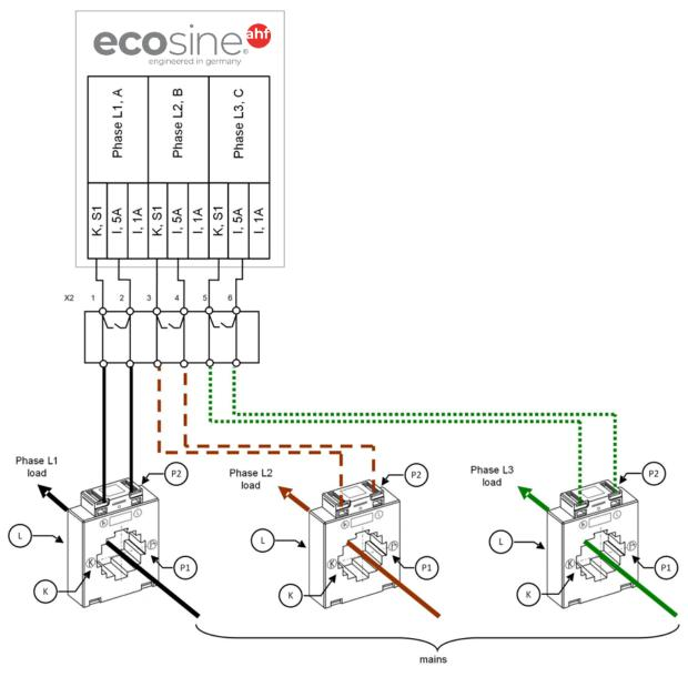
Figure 8-17 CT (5A) wiring for the sync module
