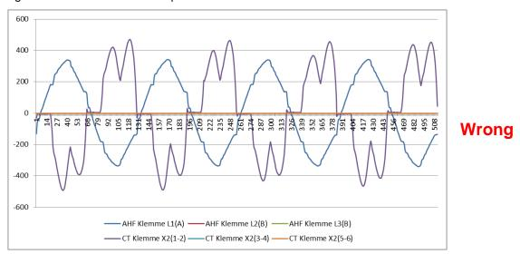
Figure 8-27 Phase of current and voltage is shifted through 180°
