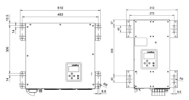
Figure 7-3 Dimensions [mm] drill-pattern for wall-mount (book and flat mounting)
