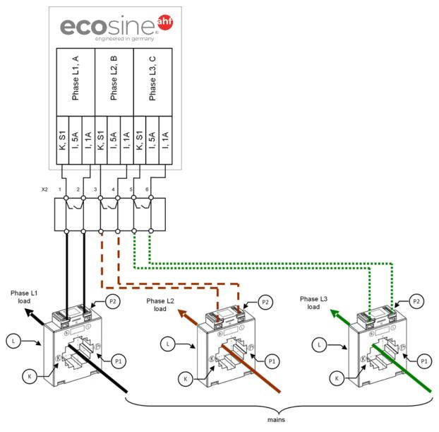
Figure 8-18 CT (1A) wiring for the sync module
