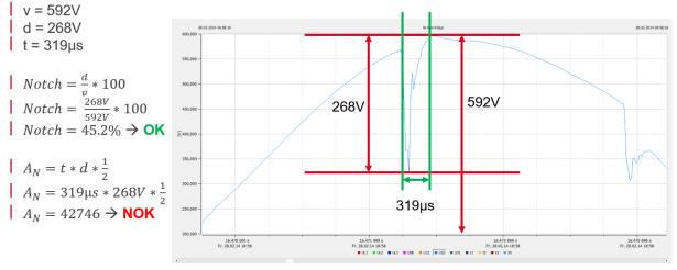
Figure 19-5: Example of notch calculation where notch depth is OK, but commutation area is NOK. These notches are not acceptable.
